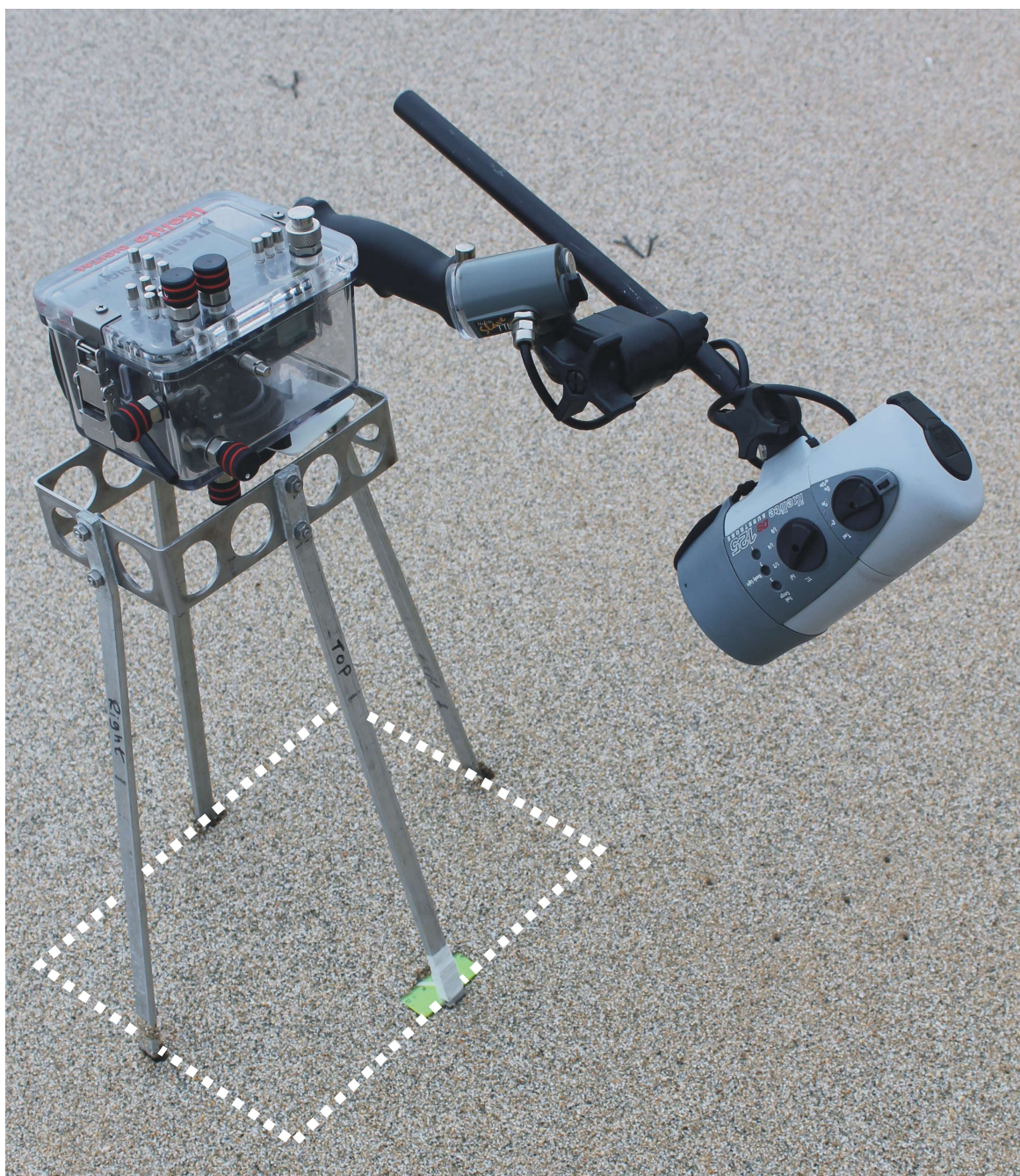
Figure 7. Waterproof housing for digital camera with attached quadrate-framing device. The dotted white line is superimposed on the photograph to indicate the perimeter of each photo-quadrate (30.5 x 22.8cm).
