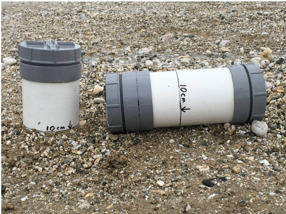
Figure 9. Hand-held coring device used in this study for sampling benthic sediments and associated macrofauna. The corer on the left is buried to the required depth for sampling. The corer on the right has been capped to retain a sampled core.
